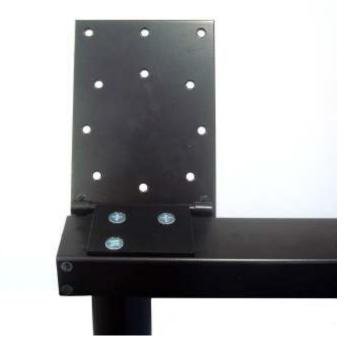
Step 4: Attach the center hinge with release handle to steel beam. Use a 3/16" Alan wrench and the provided hex head bolts to attach the hinge to the steel beam.
